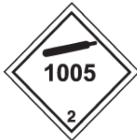
Placard for UN1005, ANHYDROUS AMMONIA
